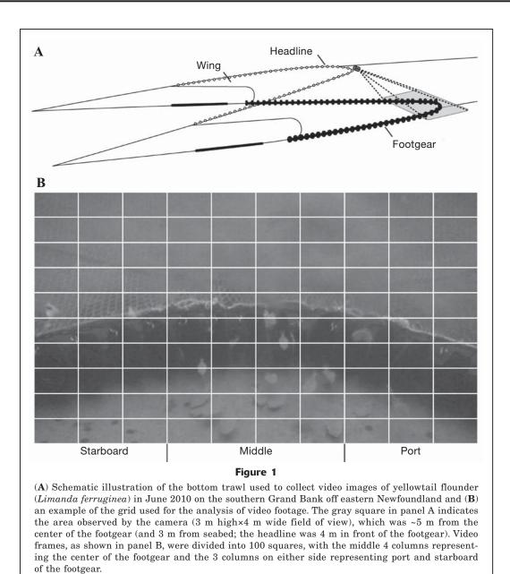
and durations of tows were in a range of 2–3 h. Tow direction was decided by commercial operations and was different for each tow. The height of the headline was approximately 3 m and was recorded with a sensor (Marport Stout Inc., Snohomish, WA) attached to the headline on all tows without the use of camera documentation during the cruise. The door spread ranged from 113 to 123 m and was measured with spread sensors (Marport Stout Inc.) placed on the trawl doors.
