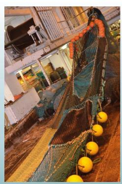
Figure 3.7. Floats mounted on both sides of the rubber mat. In addition to camera observations, the performance of the ExFED was verified by comparing the catch rates during twin trawling: one trawl with and one trawl without ExFED.
