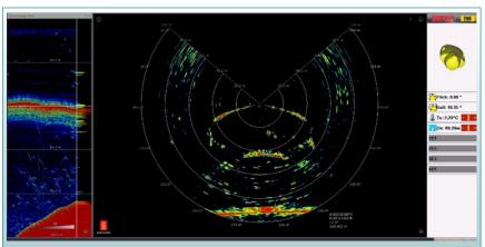
*Figure 2.3.* Display from a multibeam trawl sonar used on a pelagic trawl.
