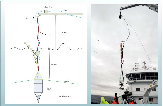
*Figure 2.2.* Set up for deploying the monitoring platform from the fishing vessel using a crane.
