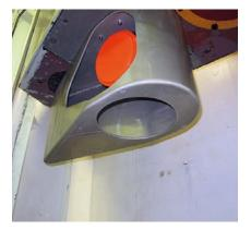
Figure 1.1. The new transducer mounting on board G.O. Sars, November 2014.
