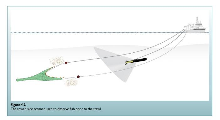
passing the camera positioned in front of the codend. While on the "G.O.Sars", the use of a towed side scanner was tested to observe fish behaviour prior to entering the trawl (Figure 4.2).
