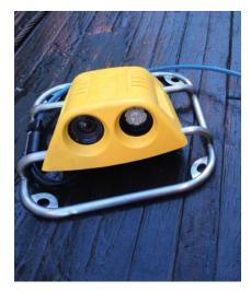
Figure 2.1. The new housing for the trawl camera.
