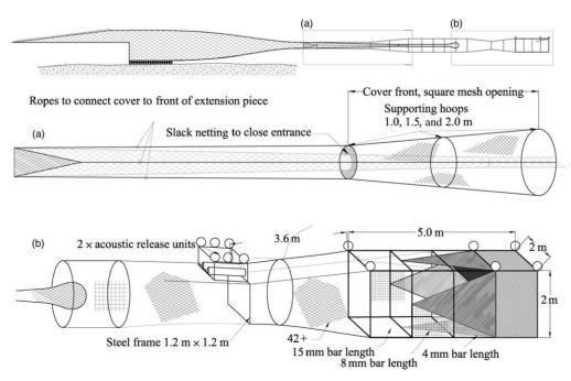
Figure 3. The attachment of the codend cover and cage to the trawl: (a) detail of cover attachment to the trawl extension; (b) detachable cage and attachment to the cover.
