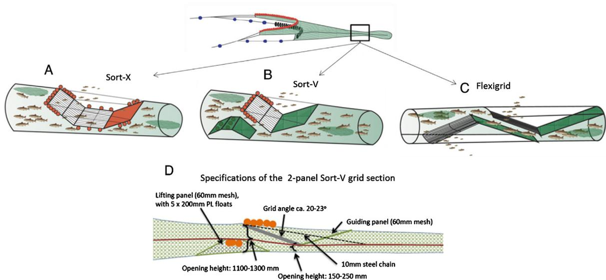
**Fig. 1.** Sorting grid sections that are mandatory in the Norwegian Sea (north of 62° N) and Barents Sea demersal fishery: (A) Sort-X, (B) Sort-V, and (C) Flexigrid. (D) Shows the specifications of a 2-panel Sort-V grid section.
