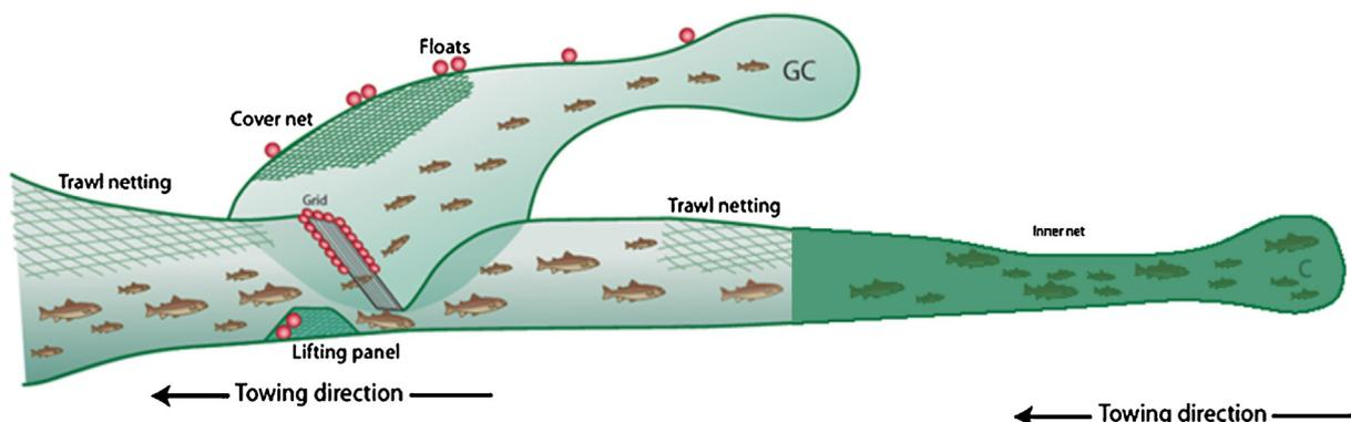
**Fig. 4.** Grid and codend setup: A grid cover (GC) collects the fish escaping through the grid, and the codend (C) is blinded with an inner net (CC).
