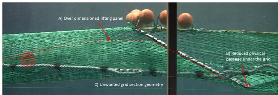
**Fig. 3.** Grid section (2-panel Sort-V) showing the over-dimensioned lifting panel that blocks the grid (A), the grid blocking the passage towards the codend (B), and the unwanted grid section's geometry as a result of using low density PE netting in the lower panel (C).
