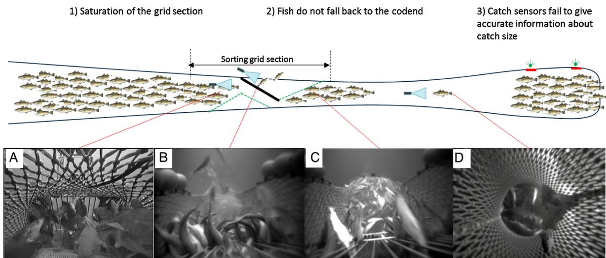
**Fig. 2.** Problems associated with current mandatory sorting grids during the fishing operation: (1) Saturation of the Sort-V grid section. Image (A) shows lots of fish swimming in front of the grid; image (B) shows lots of fish blocking the grid. (2) Fish do not fall back to the codend: Image (C) shows lots of fish swimming behind the guiding panel; image (D) shows few fish falling back to the rear most part of the codend. All images are from the tow process at 70 m depth in natural light.
