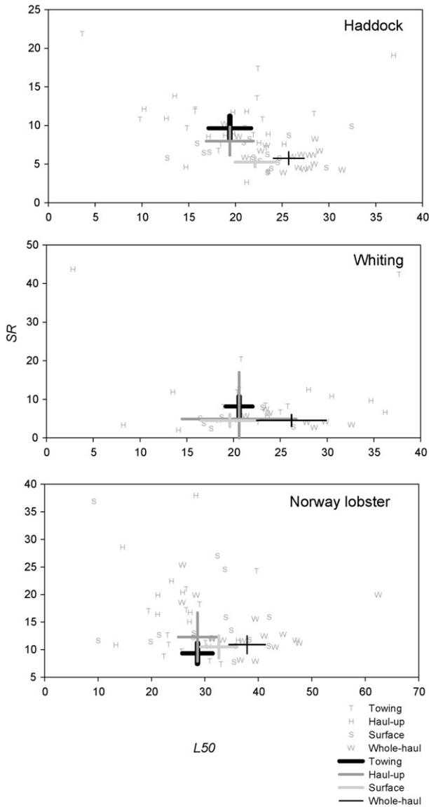
Fig. 2. Estimates of selectivity parameters for individual hauls and the mean selection curves generated by the REML analysis with lines indicating 95% confidence levels. Parameter estimates in centimetre for haddock and whiting and mm carapace length for Norway lobster.
